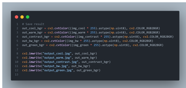
Fig. 7. Saving the transformed images after applying the different color matrices.
