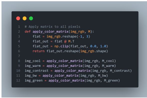
Fig. 6. Function for applying a 3 \times 3 color matrix to all pixels of the RGB image.
